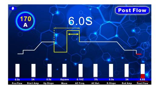
Once all settings have been set, you can start welding immediately or return to home screen by pressing home button and then you can adjust amperage or other settings if required.
