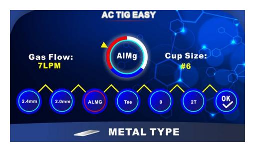
Then use control knob to select filler rod used. ALMG = 5356 Filler Rod, ALSI = 4043A Filler Rod
