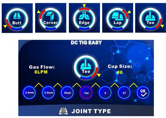
Once correct joint type has been selected, press right arrow to move to next setting.
