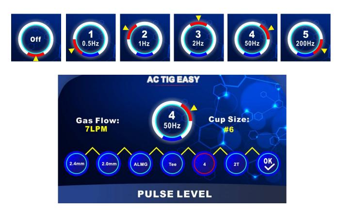
Pulse welding was designed mainly for stainless steel and other exotic materials to control heat input to the metal and decrease heat deformation.
