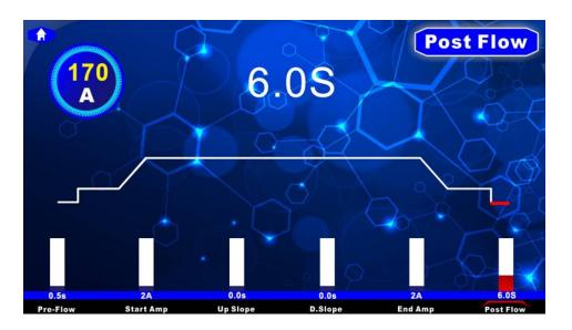
Once all settings have been set, you can start welding immediately or return to home screen by pressing home button and then you can adjust amperage or other settings if required.
