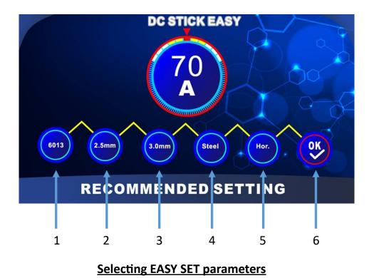
Use the left and right arrow buttons to move between each setting - once setting is highlighted in RED you use the control knob to change. Once you have entered all 5 parameters for weld, move onto OK so it goes RED (You can also press home button), the recommended welding amperage will be shown in middle of display.
